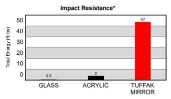
\* Instrumental Impact per ASTM D3763. Sample thickness is 0.125" nominal
